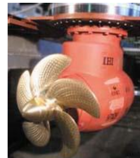
▲ Pod propulsion system with HTS motor
